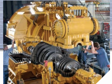
15 MW steam turbine generator set.
