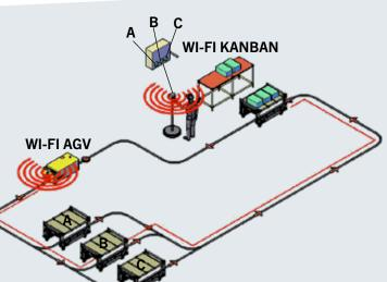
The bridge provides an interface between the AGV and the customer's system (e.g.: roller conveyors, production lines, robot, etc..). Communication of all data relative to the transfer of goods according to custom preset sequences
