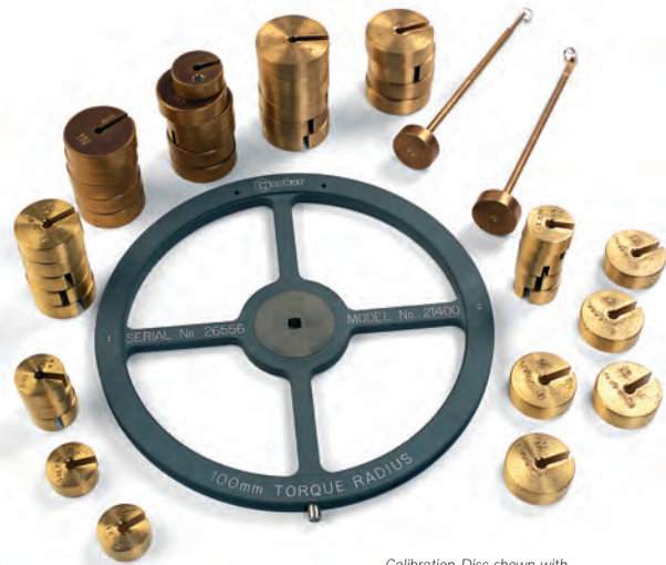
Calibration Disc shown with more than one weight set.
